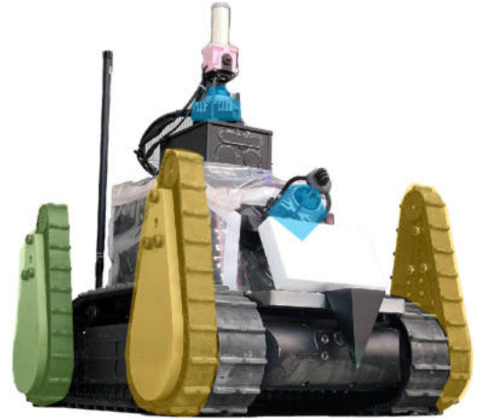
Figure 11. Slugcat: a swift articulated tracked robot for rescue missions. The orange sections represent the coaxial front flippers, the green sections represent the coaxial rear flippers, and the blue sections indicate the LiDARs.
